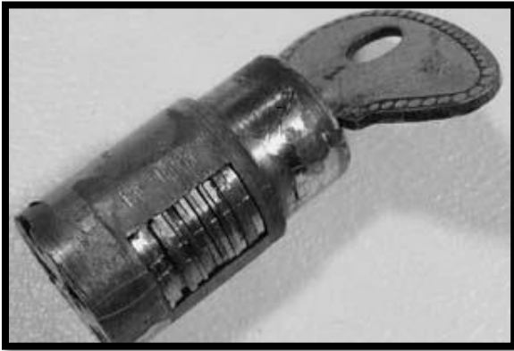
Early King lock plug and key from Briggs & Stratton ignition switch. The wafers are of three different metals of differing thicknesses. The scratch marks across the wafers are probably from the factory. The wafer pack consists of 16 wafers and uses no springs.
