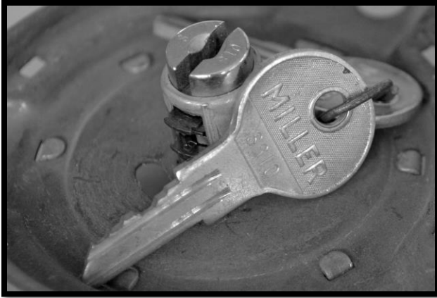
The new-old-stock Clum ignition switch above has a single-bitted Miller wafer lock with the Ilco equivalent R997N key. The key code S810 indicates its use for 1926 - 1927 Peerless.
