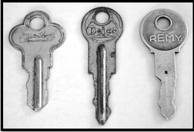
These early Yale, Delco and Remy double-bit keys were for 4-wafer automobile locks.
