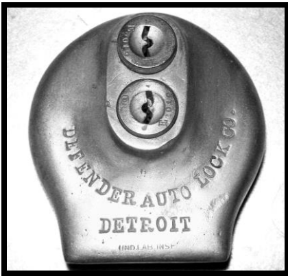
This Defender Auto Lock, an aftermarket lock for 1914 - 1918 Ford Model T, used two early King locks, one for the ignition switch, the other locking the coil case.
