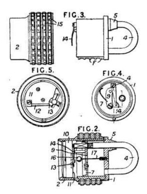
stop the watch, indicating the time of securing the padlock, the hands of the watch being visible at the outer end of the member 2. To release the padlock, the members 1, 2 are separated by setting the correct combination and the catch 9 released to free the shackle. The watch is made of non-magnetic material or guarded against retardation by means of a magnet. A ball 16 is held in the lock by a thin filament 17 so that any
